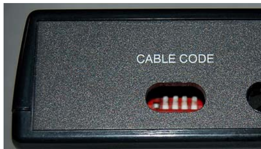
Figure 80 - Cable Code Switch (#1 shown)
