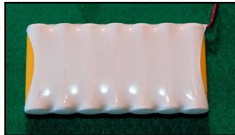
Figure 45 – Nickel-Cadmium Battery with no accessible cell terminals
