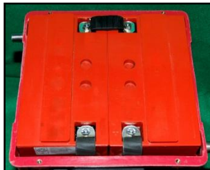
Figure 48 – SLA Battery with accessible blocks
